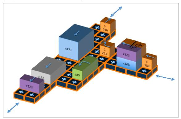
Figure 5.  $\pi$  -conveyor grid composed of flexible conveying  $\pi$  -cells
